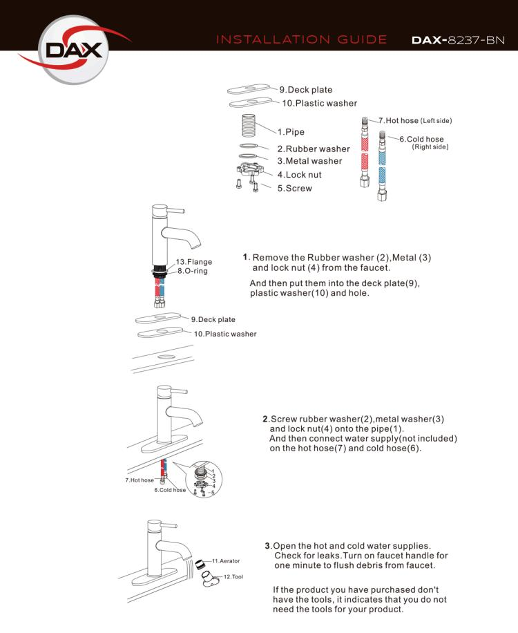
If water flow is too small or no water, the aerator may be blocked. If so, you should use the tool(12) to take off the aerator(11), clean it and re-install it.
